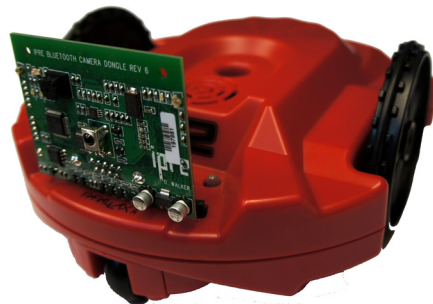
The Scribbler robot with the Fluke Dongle.
